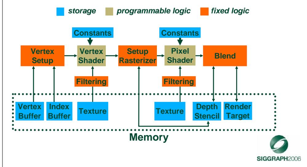
This represents the main functional units in the GPU pipeline as it exists today. The Xbox 360, the Playstation 3 and current PCs all share this GPU architecture. For the purposes of this talk, we are most interested in the two programmable shader units. Currently there is a programmable vertex shader or vertex program, and a programmable pixel shader or fragment program. The rest of the pipeline is fixed-function (but highly configurable) logic.
