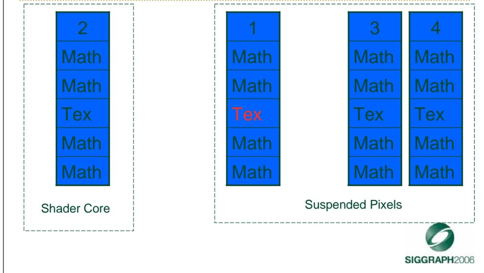
When the GPU hits the Texture instruction, it halts the pixel thread, and puts it in the suspended pixels. The program counter and register state is halted at that texture instruction. Shader instance 2 is now loaded into the core.
