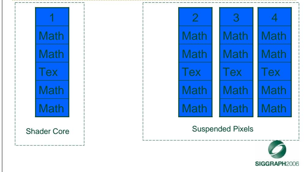
In this theoretical GPU, we have one shader core and 3 suspended pixels. The shader core starts by executing shader instance #1, which corresponds to a specific pixel on the screen.
