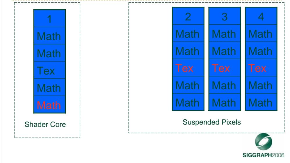
Finally, the shader core reloads pixel #1, and the texture load data should now be ready, having been sent across the bus
