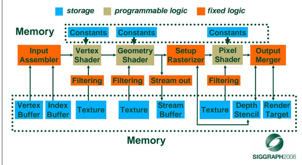
This shader model is the one exposed in Direct3D 10. Hardware supporting this model should be available in late 2006. Most of the differences from shader model 3 are related to memory access, however the introduction of the Geometry Shader fundamentally alters the kinds of shading which can be performed, since shading is now possible at the triangle level if desired.
