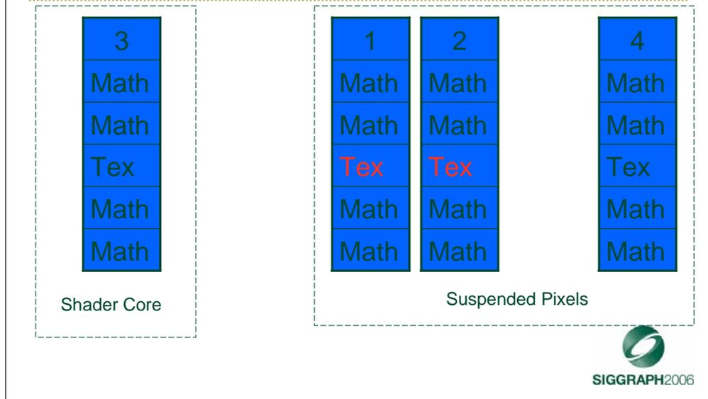
Now, shader instance 3 is loaded into the shader core, and executed until the texture instruction.
