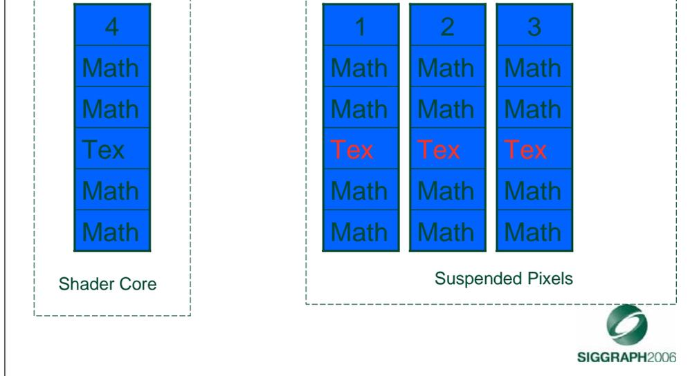
Finally, the shader core gets to pixel instance #4, here we have 3 partially executed pixels waiting to be completed.
