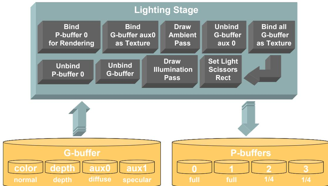
**Figure 5:** Lighting stage of deferred shading general architecture.
