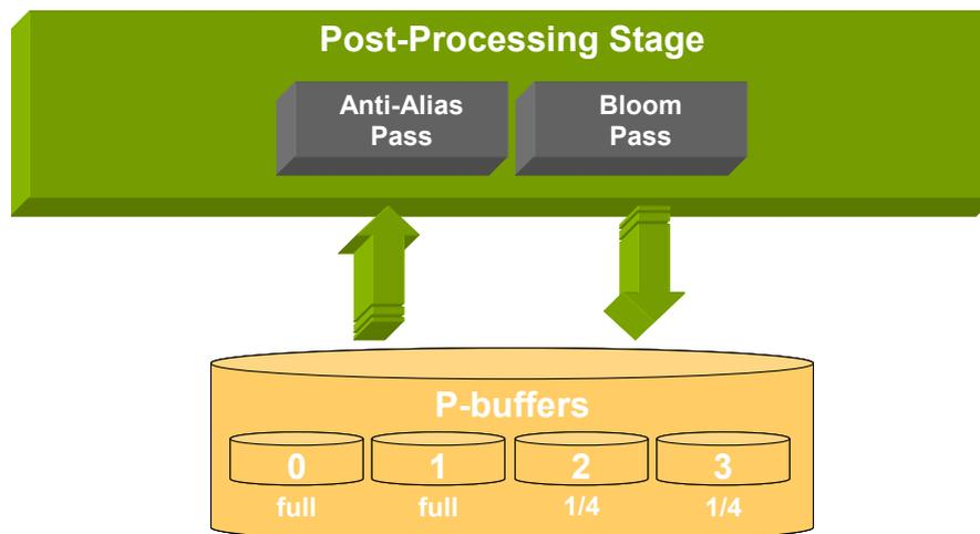
**Figure 7:** Post-processing stage of deferred shading general architecture.
