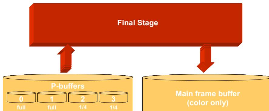
**Figure 12:** Final stage of deferred shading general architecture.
