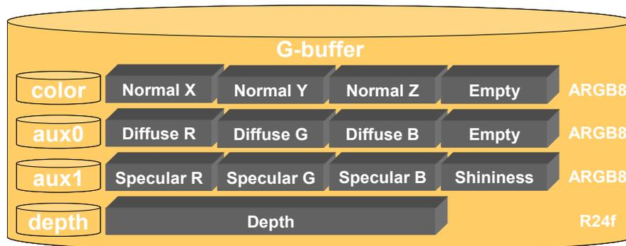
**Figure 3:** G-buffer configuration adopted in the implementation of the deferred shading technique presented in this tutorial.
